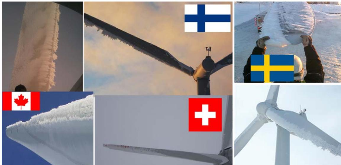
Figure 2. Icing on wind turbine blades in different parts of the world (source: Task 19)
