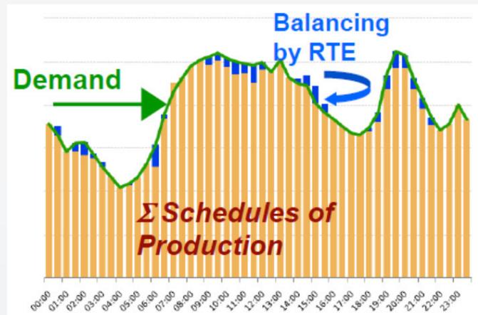
Figure 3. Scheduling the generation units is made to cover the anticipated demand, at least one day-ahead. Dispatch can be fine-tuned closer to real time. During the operating hour, balancing (operating reserves) are used to maintain the balance—load following by manual dispatch and automatic regulation in some power plants to follow the second to minute variability. (Source: RTE, the transmission system operator of France)
