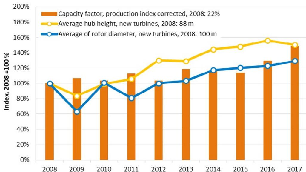
Figure 2. Growth of turbines built in each year and development of average capacity factor of all wind turbines in Finland, 2008-2017
