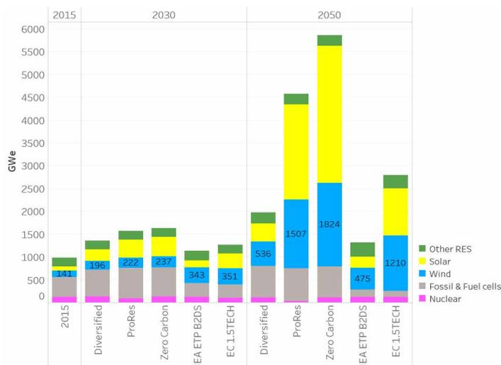
Figure 4. Installed generation capacities in the EU by 2050 for different decarbonization scenarios of the JRC-EU-TIMES model, as well as for the IEA ETP B2DS and EC 1.5TECH scenarios [2-4, 6]
